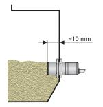
Sensing bulk-solid materials in storage tanks
